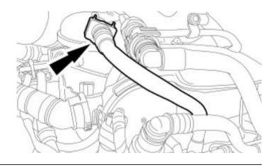
Install one end of a suitable hose onto the secondary fuel filter and the other end into a suitable container.
